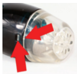
2 - 5 Push a Pen into the Right-Hand Side of the Window. Twist Cap Counter-Clockwise and Lift the Cap Clear
